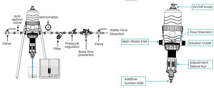
Fig. 2 - Installation illustration
